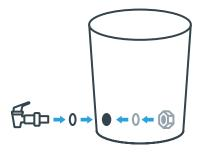
Place the water tap assembly and one gasket through the hole drilled on the
