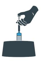
Back wash filter using only clean water and syringe until water runs clear
