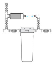
Place rubber tubing over barbed end of secondary filter on one end and over barbed nub of the water output assembly on the other end.
