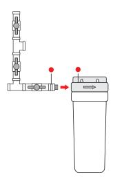
Locate red dot on filter input and red dot on water input assembly. Wrap supplied teflon tape around threaded end of water input assembly 2-3 times to prevent leakage, then screw water input assembly onto filter input.
