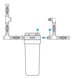
Locate blue dot on filter output and blue dot on water output assembly. Wrap supplied teflon tape around threaded end of water output assembly 2-3 times to prevent leakage, then screw water output assembly onto filter output.
