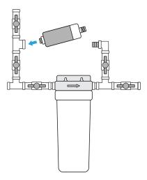
Screw secondary filter into the receptacle on the water input assembly.
